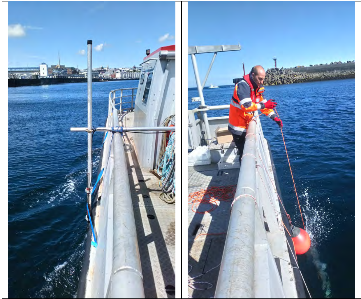
Figure 3. ADCP mounted to port side of vessel (left) and water sampling (right)
